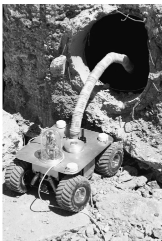
Figure 1: A mobile search and rescue robot. Taken from Figure 1 of "Design and control of a mobile hyper-redundant urban search and rescue robot" by Wolf et al.
